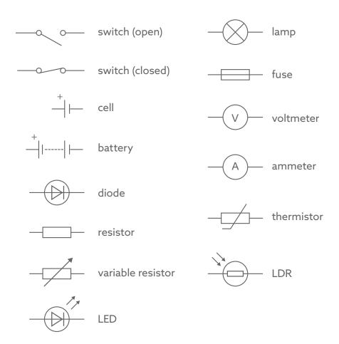
Students should understand the use of thermistors in circuits, for example thermostats.
